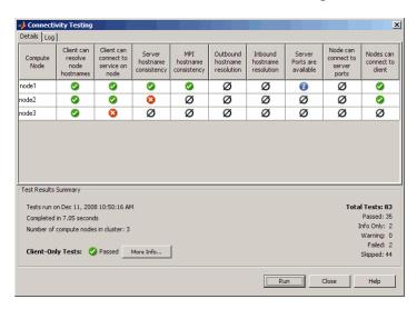
Double-click any of the symbols in the test results to drill down for more detail. Use the **Log** tab to see the raw data from the tests.
